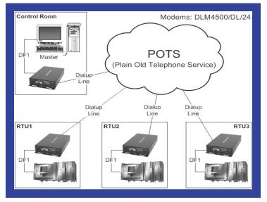
Diagram 1. A typical dial-up communication system where the control room computer dials each RTU to establish a temporary point-to-point session.
