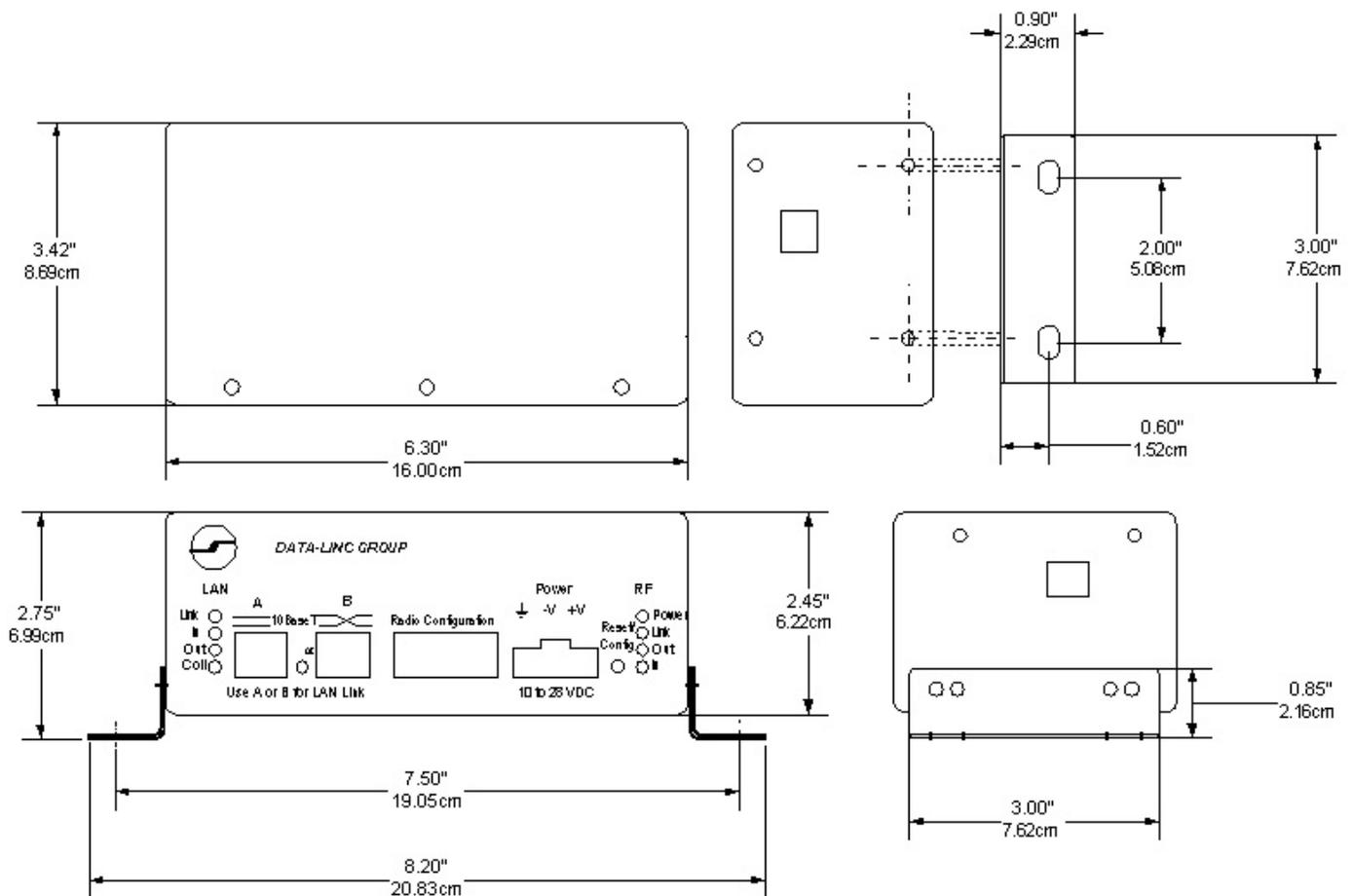
**Note:** Enclosure Size, Mounting Holes and Locations may change without notice, contact Data-Linc Group (425) 882-2206 for the latest Enclosure Dimensions.
