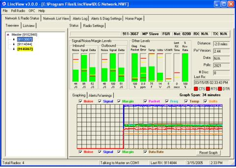
The following illustrates an alarm in the Radio Status tab.
